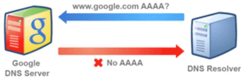
...but a DNS resolver with Google over IPv6 will receive an IPv6 address, and its users will be able to connect to Google web sites using IPv6
